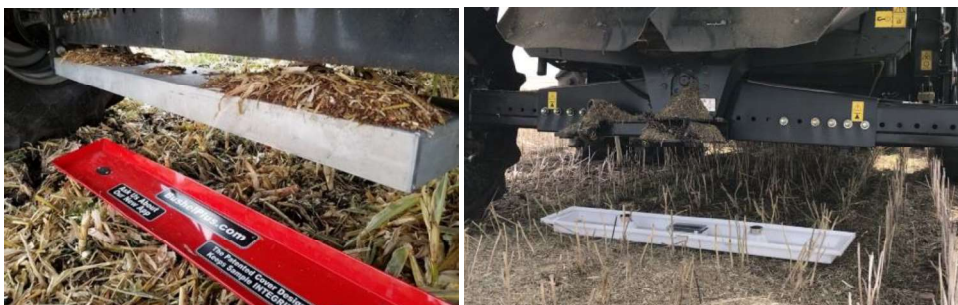
Figure 3. Bushel Plus drop pan (left; image source: http://bushelplus.ca/bushel-plus-harvest-loss-system/ ) Schergain drop pan (right; image source: https://www.schergain.ca/pricing/ ).
