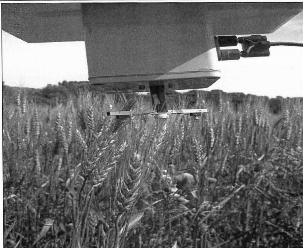
Figure 3. Rotorod spore trap in the wheat strip.
