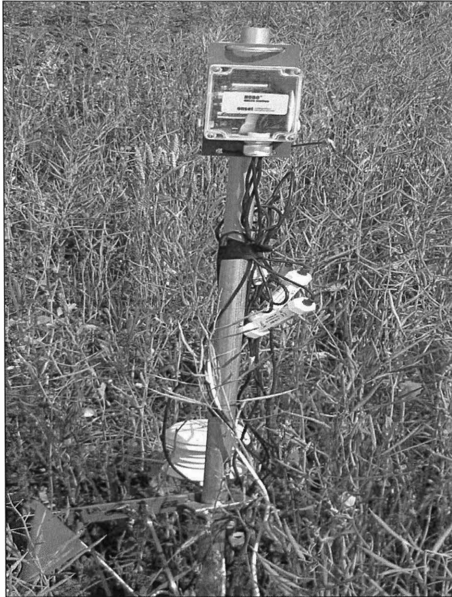
Figure 2. Microclimate station deployed in a canola plot.
