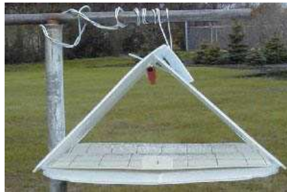
Figure 4 Sticky bottom placed in trap
