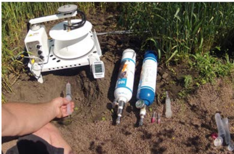
Figure 2. Measuring N 2 O with FTIR instrumentation in field, Saskatoon, SK.
