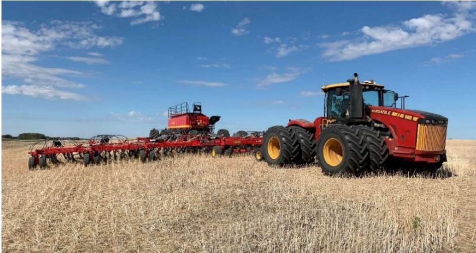
Figure 3. Versatile tractor and Seed Hawk Vaderstad implement and cart.
