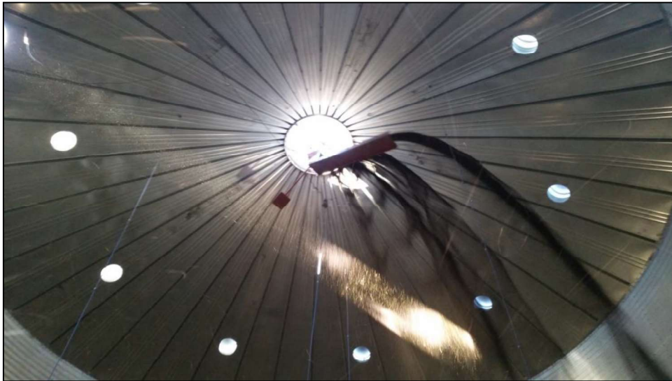
Figure 4. ‘Gravity-driven’ spreader (as viewed from the bottom).
