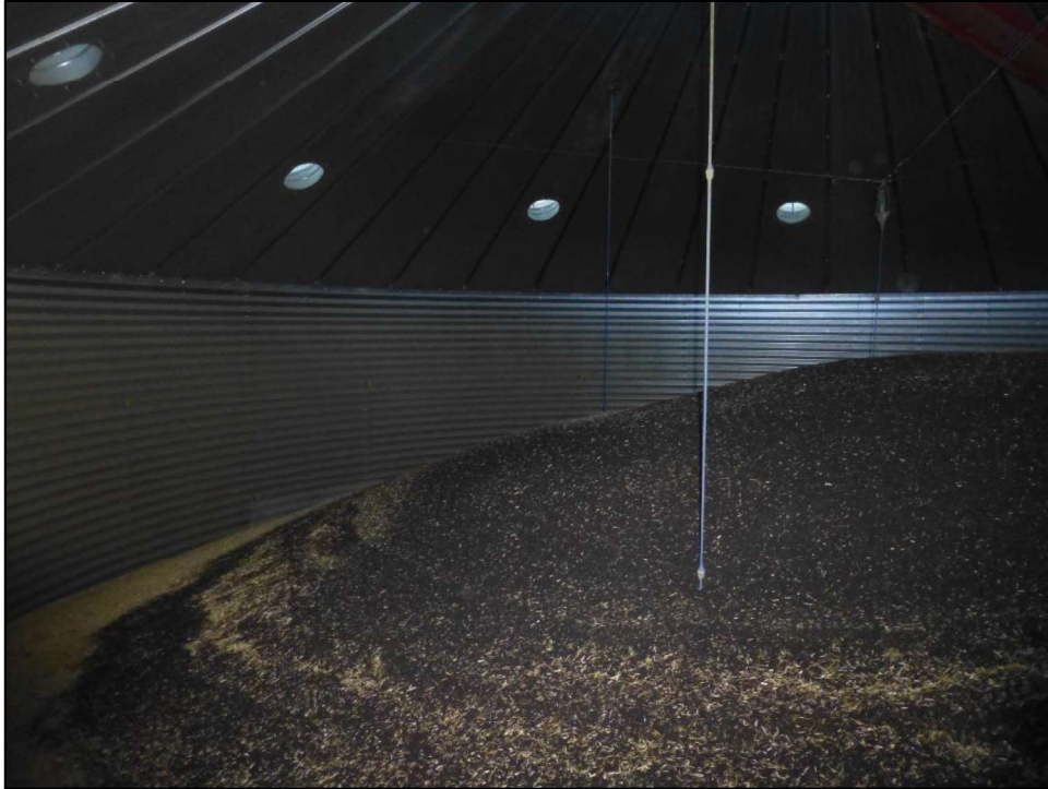
Figure 11. Grain profile from inside the bin when filling with the spreader.
