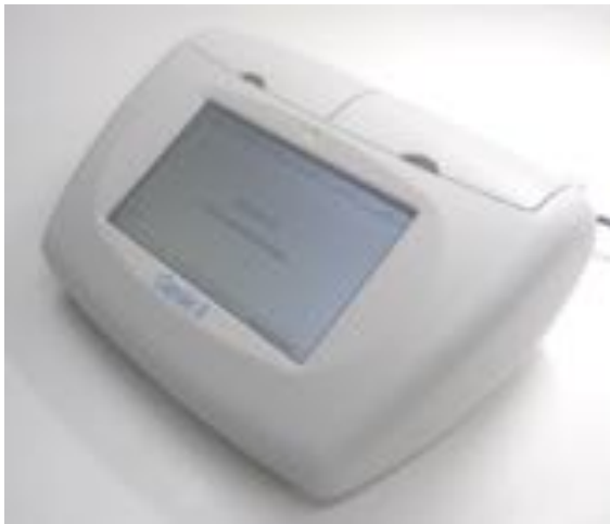
The visual detection Real Time PCR Detection System or Genie® II
